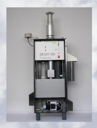
PM10- and PM2,5 STANDARD REFERENCE SAMPLER according to CEN EN 12341
